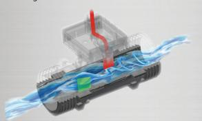
All Torus Series come standard with a Sika flow switch. Units are also available with an optional SIKA vortex flow sensor mounted in a by-pass configuration and mapped to indicate the boiler flow in (gpm). The SIKA flow sensor utilizes vortex technology which is then converted to an electrical signal sent directly to the HeatNet Boiler Management System for real time flow annunciation. The SIKA flow sensor is fully adjustable throughout the operating range.
